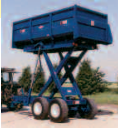
HL10 10 tonne capacity high lift trailer with extension chute
