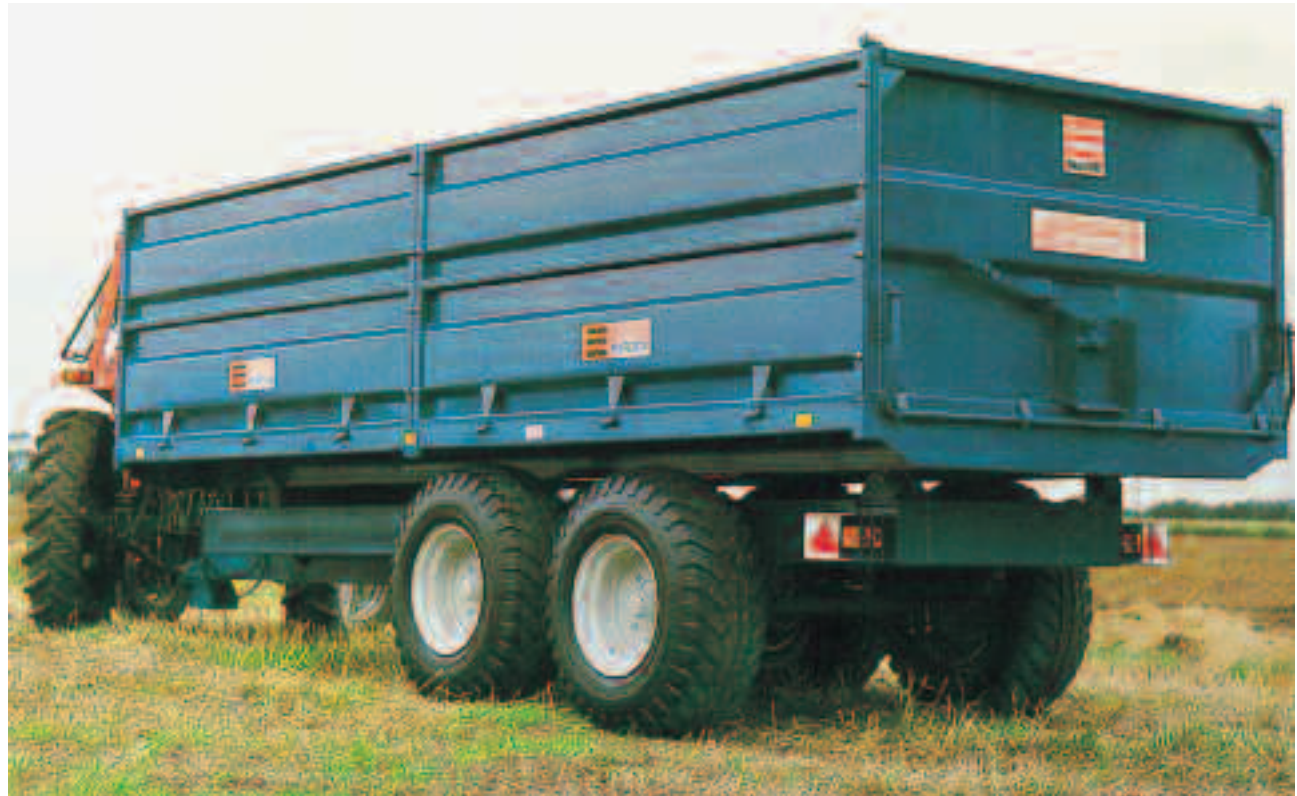
D12 12 tonne grain trailer fitted grain chute
