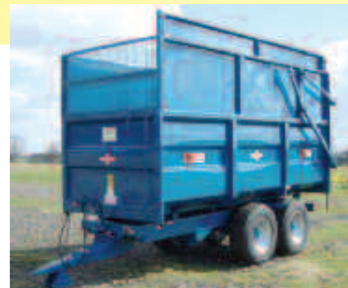
ACE11 fitted optional sprung drawbar side load silage auto up-over-door
