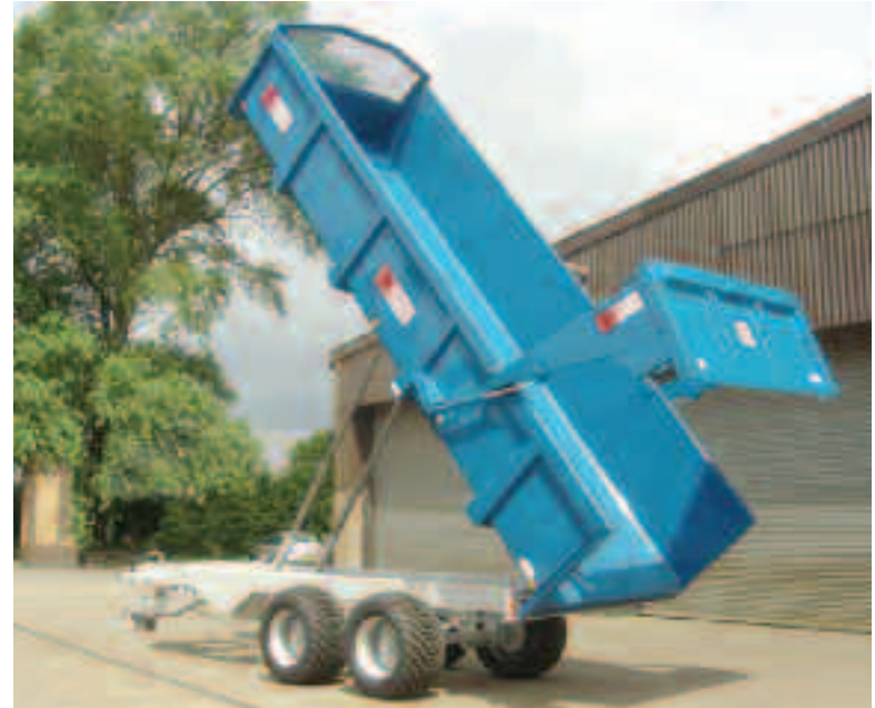
RCT14 basic trailer fitted optional flotation tyres
