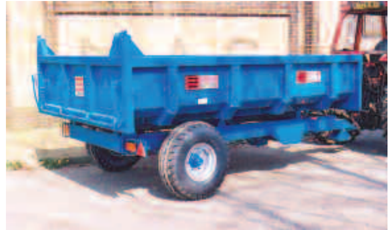
SRT 6.5 tonne stone and rubble trailer
