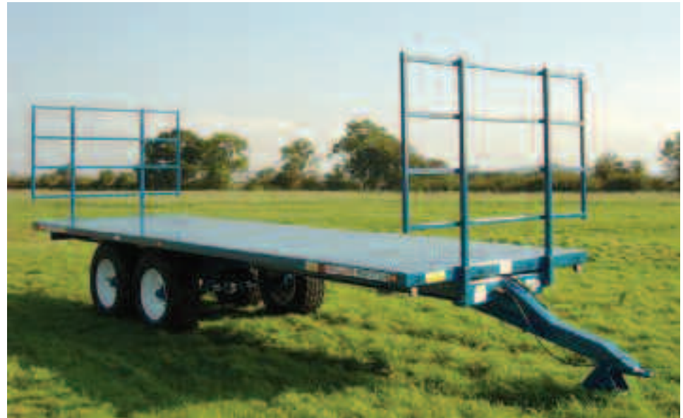
BT10 10 tonne capacity fitted 385/65R 22.5 tyre
