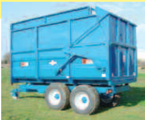
ACE10 fitted 385/65 remould tyres hydraulic tailgate combination silage
