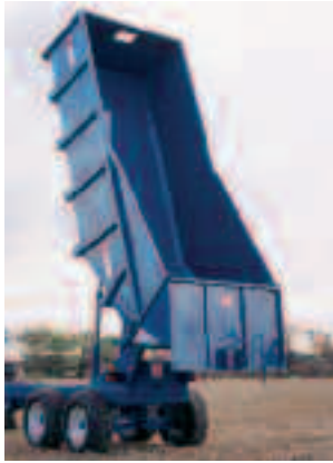
Ag 14 dump trailer fitted optional grain conversion kit, with grain chute and floatation tyres
