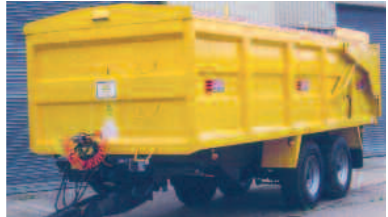
FT 180 14 tonne fitted hydraulic tailgate and roll over sheet
