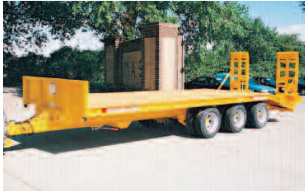
MPT22 22 Tonne capacity beavertail low loading trailer
