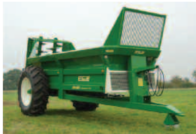
ELFM1000 10 tonne twin vertical beater manure spreader
