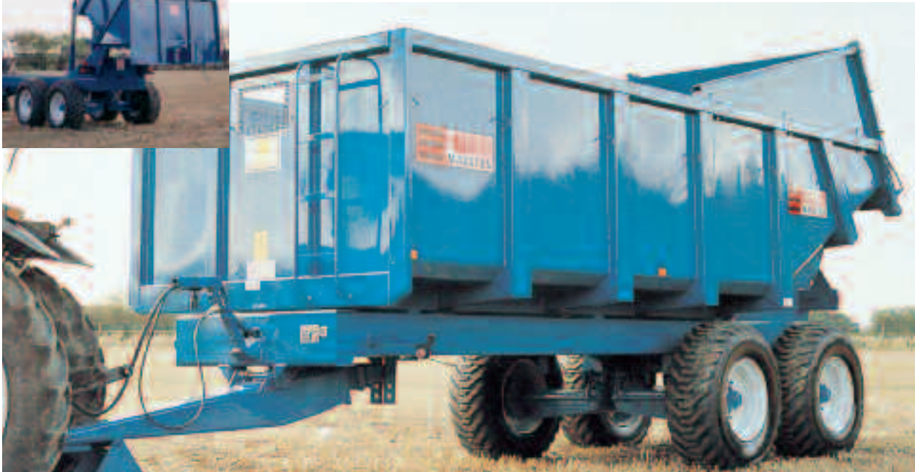
14 ton dump trailer grain conversion kit full sprung drawbar
