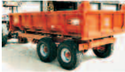
SRT 6.5 tonne stone and rubble trailer
