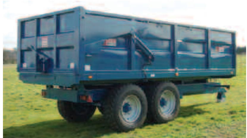
LS12 12 tonne lift-off side fitted hydraulic tailgate
