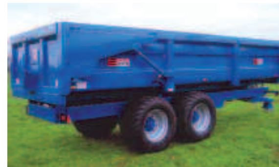
Fenlander 12 fitted hydraulic tailgate, sprung drawbar and flotation tyres
