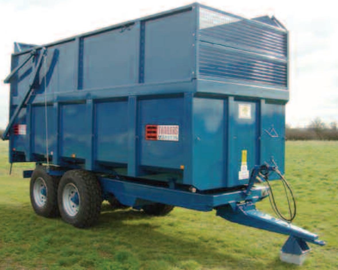
Contractor 12 side load silage auto up-over door and sprung drawbar (splatter panel non standard)
