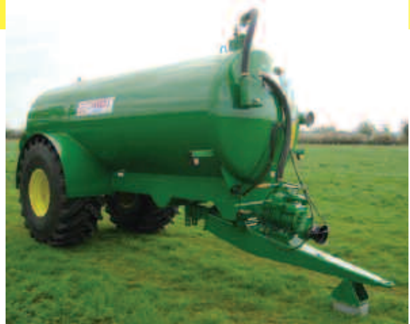
VT2000 2000 gallon single axle fitted 28.1R26 tyres and sprung drawbar
